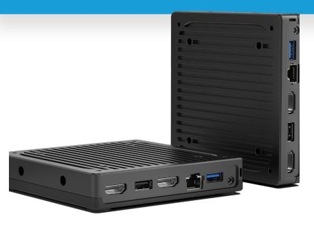
Meet the Element MPC1 Mini Box PC, a powerhouse digital signage player packed in a small form factor sleek design. Integrated with the Intel® Elkhart Lake J6412 processor, the MPC1 provides a computing experience that surpasses expectations.
